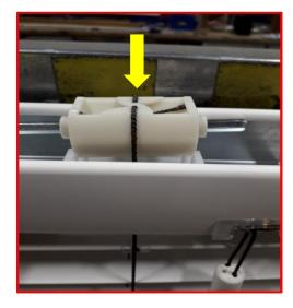
Make sure that the installation brackets are not obstructing the movement of the ladders/tapes.
