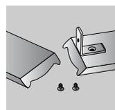
2. To fit the valance returns (if required) peel the back off the double sided tape on the fascia return bracket and place centrally into position on the valance.
