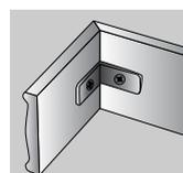
4. Make sure the corner join is satisfactory and secure using the screws supplied. Alternatively, a suitable mitre adhesive can be used.
